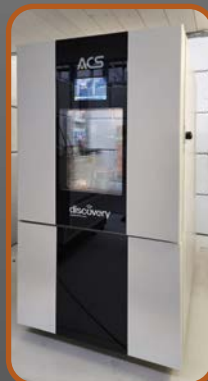
Climatic Chamber suitable for PR2F and TAT Tests
